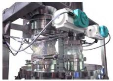
The Rotary Valve is supplied with a position feedback device that will work in conjunction with a servo pneumatic valve for optimal batch control. This allows for precise oscillation of the Rotary Valve via HMI for
