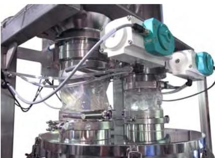
The Rotary Valve is supplied with a position feedback device that will work in conjunction with a servo pneumatic valve for optimal batch control. This allows for precise oscillation of the Rotary Valve via HMI for highly accurate batching while minimizing wear and tear on the valve seal.
